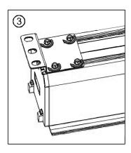
Tighten the bracket nuts. This will ensure the screen does not slide or vibrate during installation.
