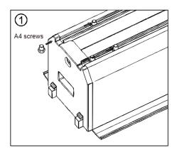
Slide 4 of the screws (A4) into the rail located on top of the screen.
