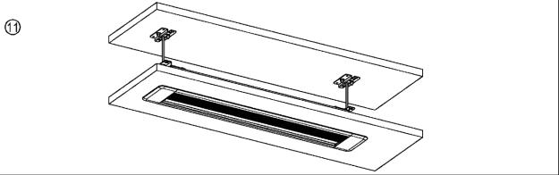
The screen installed should leave no gaps in the ceiling as shown.
