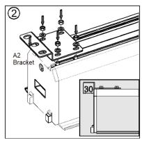
Install the screen bracket (A2) while leaving 30mm out from the edge of the screen.
