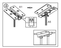
Attach the threaded mounting rod (A5) to the ceiling bracket (A1) on the top and bottom of the bracket using the M10 nuts and washers provided.
