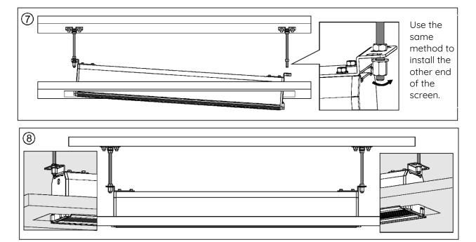
Adjust the position of the screen after hand tightening all the nuts. Leave as little gap as possible.
