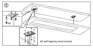
Use the A8 anchor bolt for a concrete ceiling or the A6 self-tapping screws for a wood ceiling. Attach the A1 bracket to the ceiling in the desired location. It is highly recommended that you provide your own ceiling screws/hardware for any other materials/surfaces you wish to mount the screen onto.
