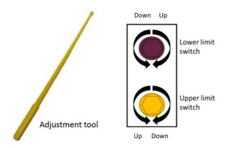
The limits that are set determine the point at which the screen will stop lowering or retracting. By initially adjusting the lower limit, the screen will stop at the perfect location automatically for maximum convenience.
