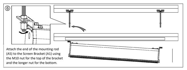
Be sure to leave enough space so the bracket can move when installing the other end.
