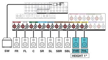
\* The rear height speakers can be connected instead of the front height speakers. In this case, set the height speakers to be connected under "Height" - "Layout" in the menu. (② p. 227)
