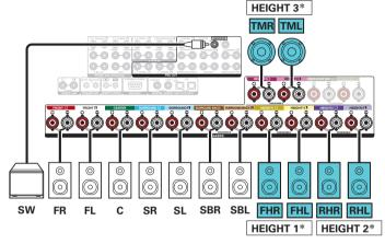
\* You can change the combination of the HEIGHT1, HEIGHT2 and HEIGHT3 channels in the settings. (@p p. 69)
