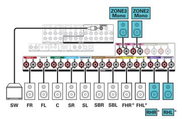
\* The height speakers, ceiling speakers and Dolby Atmos Enabled speakers can be connected to the HEIGHT1 and HEIGHT2 speaker terminals. Set the speaker to be connected from "Height" in the menu. ((இ) p. 225)
