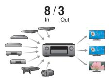
For connection to a broad range of digital sources, this unit features 8 HDMI inputs, including 1 on the front panel that lets you quickly and conveniently connect a camcorder, game console or other HDMI-equipped device. There are dual HDMI outputs for the main room, and a third HDMI output for another room.
