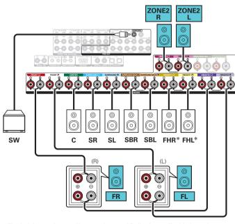
\* The height speakers, ceiling speakers and Dolby Atmos Enabled speakers can be connected to the HEIGHT1 and HEIGHT2 speaker terminals. Set the speaker to be connected from "Height" in the menu. ((27) p. 225)
