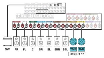
\* The top front or top rear speakers can be connected instead of the top middle speakers. In this case, set the ceiling speakers to be connected under "Height" - "Layout" in the menu. ( p. 227)
