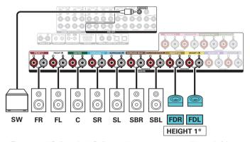
\* The surround Dolby or back Dolby speakers can be connected instead of the front Dolby speakers. In this case, set the Dolby Atmos Enabled speakers to be connected under "Height" - "Layout" in the menu. ( ) 227)
