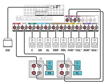
\* The height speakers, ceiling speakers and Dolby Atmos Enabled speakers can be connected to the HEIGHT1 and HEIGHT2 speaker terminals. Set the speaker to be connected from "Height" in the menu. ( ) 225)
