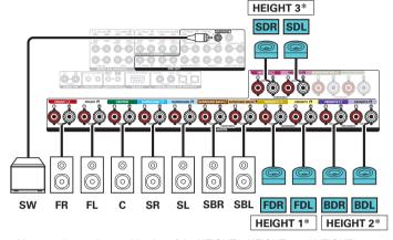
\* You can change the combination of the HEIGHT1, HEIGHT2 and HEIGHT3 channels in the settings. (127 p. 69)
