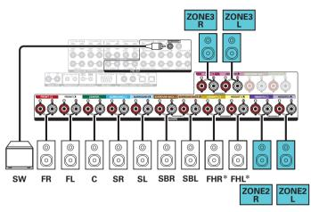
\* The height speakers, ceiling speakers and Dolby Atmos Enabled speakers can be connected to the HEIGHT1 and HEIGHT2 speaker terminals. Set the speaker to be connected from "Height" in the menu. ( ) 225)
