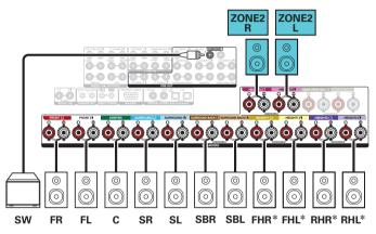
\* The height speakers, ceiling speakers and Dolby Atmos Enabled speakers can be connected to the HEIGHT1 and HEIGHT2 speaker terminals. Set the speaker to be connected from "Height" in the menu. ((27) p. 225)
